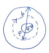
First use Ampere's Law to find the magnetic field in the coax. Align the coax on the Z axis with a current I flowing in the + az direction. This systen cylindrical symmetry
